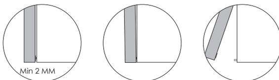
**3** MIT DER HINTEREN SCHRAUBE VOM SCHARNIERBOCK KANN DIE FRONT DEM KORPUS ANGEGLICHEN WERDEN
